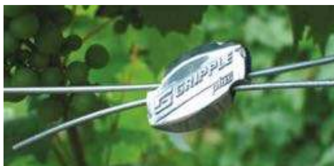
Top. Wire repair using Gripple Plus Medium. Bottom. Standard join.
