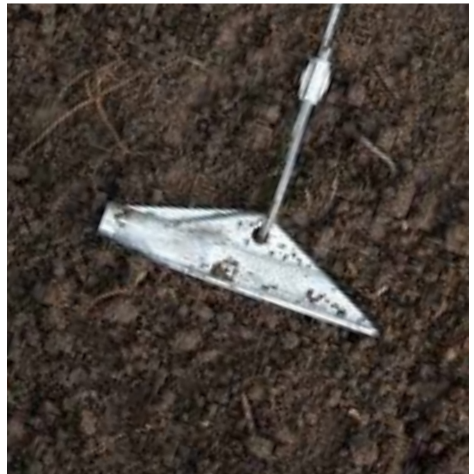
Anchor 3 - Activated and installed.
